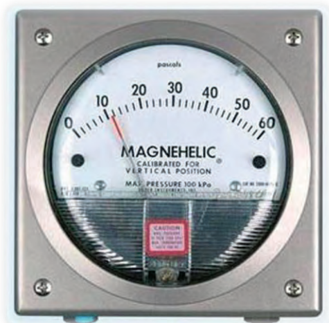
Figure 26 - A Magnahelic Pressure Gauge
