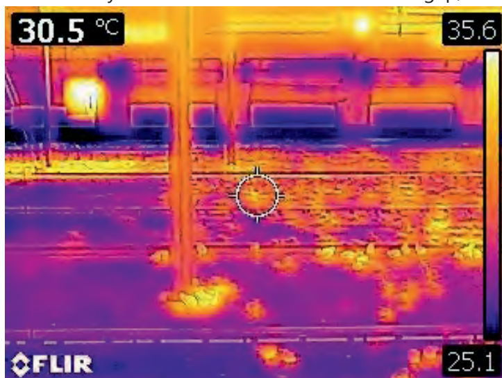
Figure 30 The same farm again gaps where it's cold on the floor the chicken will avoid it
