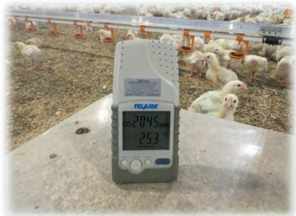
Figure 36 My Co2 Telaire handheld monitor used for farm visits (plus a nosy chick!)
