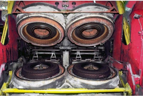
Tire molding machine. Encik Tekateki/ CC-BY-SA-4.0
