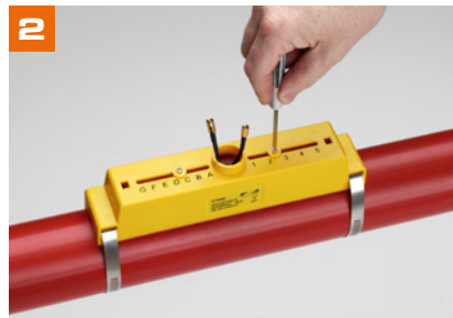
Clamp guide rail and sensor assembly to pipe and release sensor locking screws
