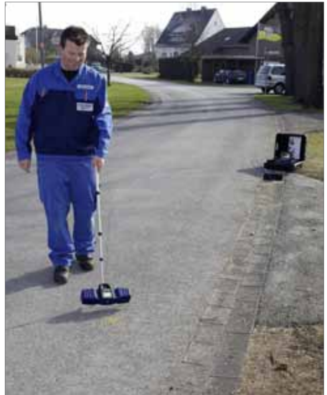
The Wöhler VIS 350 precisely locates radio waves transmitted by the camera head through concrete and asphalt to save a lot of time and further building damage.
