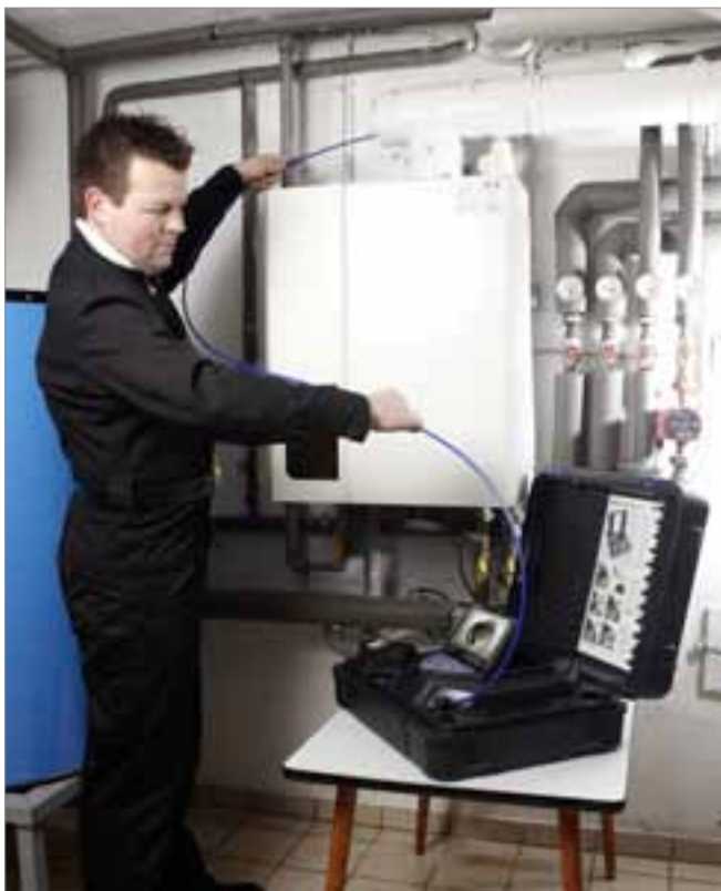
The 360° pan and 180° tiltable color camera head easily negotiates 87° bends.
