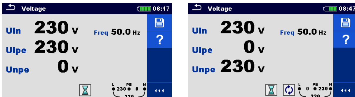
Figure 7.4: Examples of Voltage measurement in single-phase system
