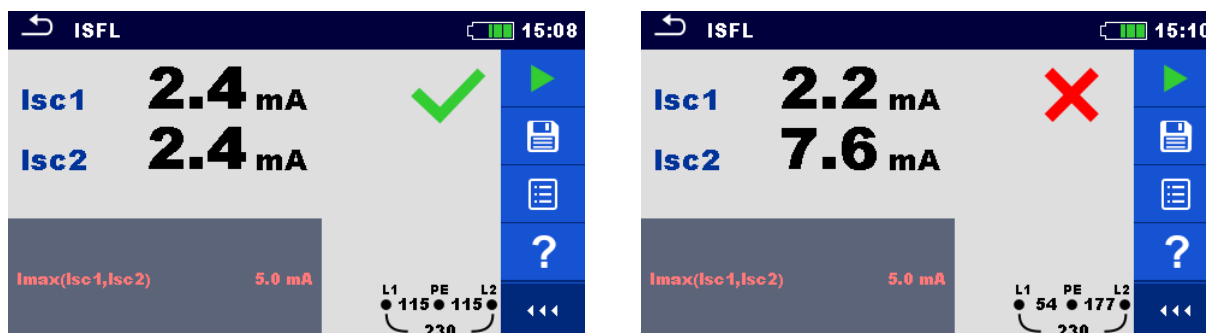
Figure 7.78: Examples of First fault leakage current measurement result
