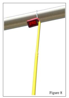
Accurate measurement of electric fields in combination with intelligent compensation for the transmission voltage effects mentioned above allows not just detection of voltage but a display of the measure of the voltage. Seen in figure 8, this new ability in a tool with a single point of contact allows users to easily distinguish nominal line voltage from induced voltage and to do so on systems up to 765kV.
