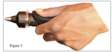
into the small distance between this hand and an inner electrode. Collapsing the very weak electric field in this manner increases the field strength and allows for a high degree of sensitivity and the detection of very small voltages including those resulting from equipment that is intact and working properly but simply ungrounded.
