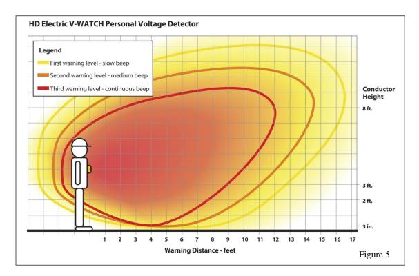
The presence of live conductors in the zone of optimum sensitivity will provide an audible and visual warning to the user from a distance of 2 to 5 meters (6.5 to 16 feet).
