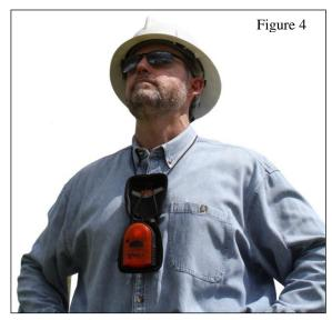
reduced sensitivity in the directions of the rear, far sides and overhead. Internal sensing electrodes exactly parallel to the plane of the body of the wearer result in optimum sensitivity in the direction of both work and movement of the user. Further shaping of these electrodes fine tunes sensitivity where it is desired and attenuates sensitivity in directions where it is not as shown in figure 5. The concentric ovals signify three distinct warning levels.
