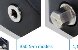
350 N·m models (43524 and 43525) supplied with ½" female square drive 1,100 N·m models (43530 and 43531) supplied with 27 mm male hexagon plus 3/4" square drive socket
