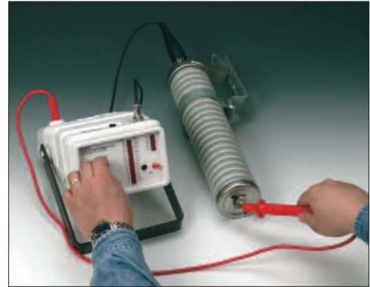
HiSat-25 testing a porcelain arrester
