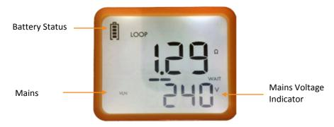
\*LCD display shown in the no trip loop function.
