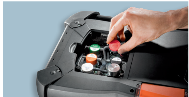
Fig. 8: testo 350 with electrochemical sensors
