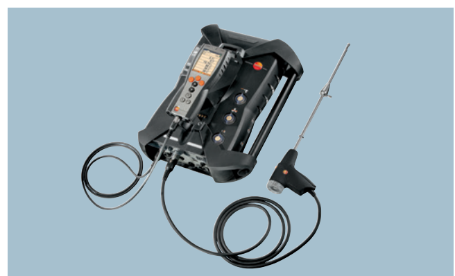
Fig. 3: testo 350 exhaust gas measuring instrument with flue gas probe
