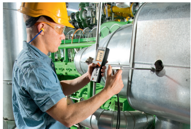
Fig. 2: testo 350 exhaust gas measurement at the engine
