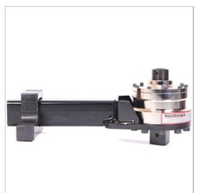
Norbar 'HandTorque' multipliers employ multiple stages of epicyclic gearing to give a wide range of torque outputs and ratios to suit most applications. Ratios quoted are always the torque multiplication ratio, not the velocity ratio as given for some competitor's products. For example, the velocity ratio may be 29.8:1 to give a torque multiplication of 25:1 ±4%.
