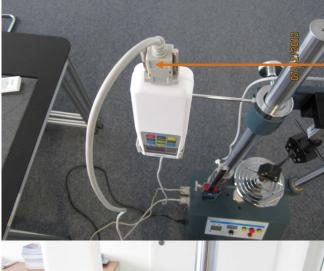
View from above FH with FH-A01 cable. A plug has to be inserted into the socket of the FH, the other one into the equipment port of TVS
