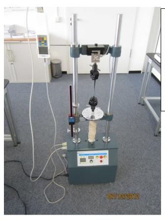
Cabling of the length measuring device:
