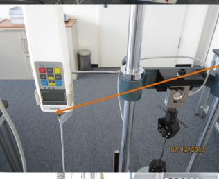
The plug of the external force gauge measuring cell has to be plugged into the socket of the FH force gauge.
