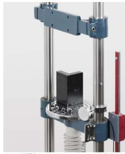
Fixing the fitting bracket AFM 41 with M6x35 Allen screws steadily with an Allen key
