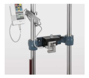
The FH force gauge mounted on the test stand now has to be connected by means of the RS232 cable with the test stand to the Equipment-Port.
