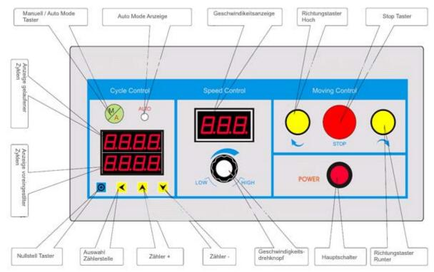
Main switch: Switching on/off the test stand
