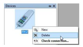
To delete one or multiple devices, select the devices to be deleted then right click within the device icon for displaying the context menu. Then select Delete. To confirm deletion, press ok in the message box.
