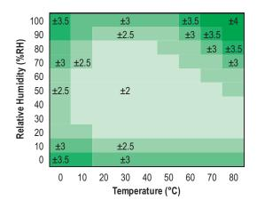
Typical accuracy of relative humidity measurements given in
