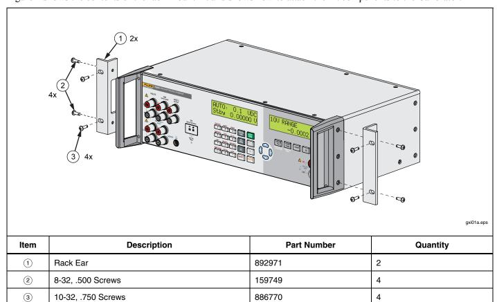
Figure 1. Attach the Rack-Mount Kit
