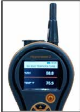
Figure 4: Hygromaster2 as a Hygrometer
