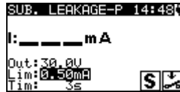
Figure 6.15: Substitute leakage - P starting screen
