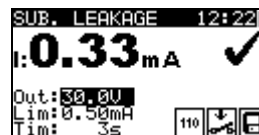
Figure 9.3: Substitute leakage screen (110 V)
