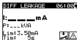
Figure 6.11: Differential leakage starting screen
