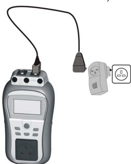
b) Testing of PRCD via mains socket
