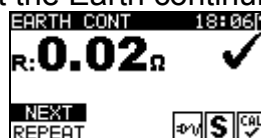
Figure 6.6: Earth continuity result screen
