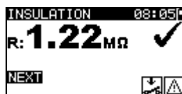
Figure 6.8: Insulation result screen
