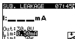
Figure 6.9: Substitute leakage starting screen
