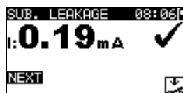
Figure 6.10: Substitute leakage result screen
