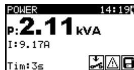
Figure 5.40: Example of apparent power measurement result
