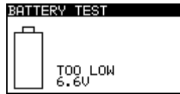
Figure 1.1: Discharged battery indication
