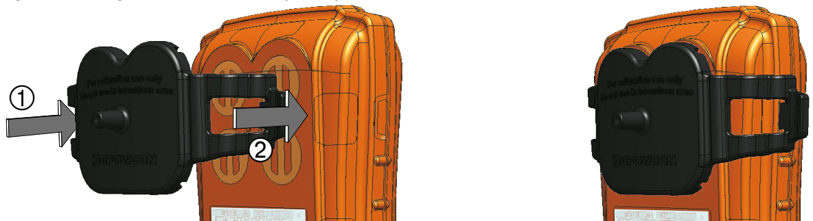
Figure 5: Fitting the calibration/bump test plate
