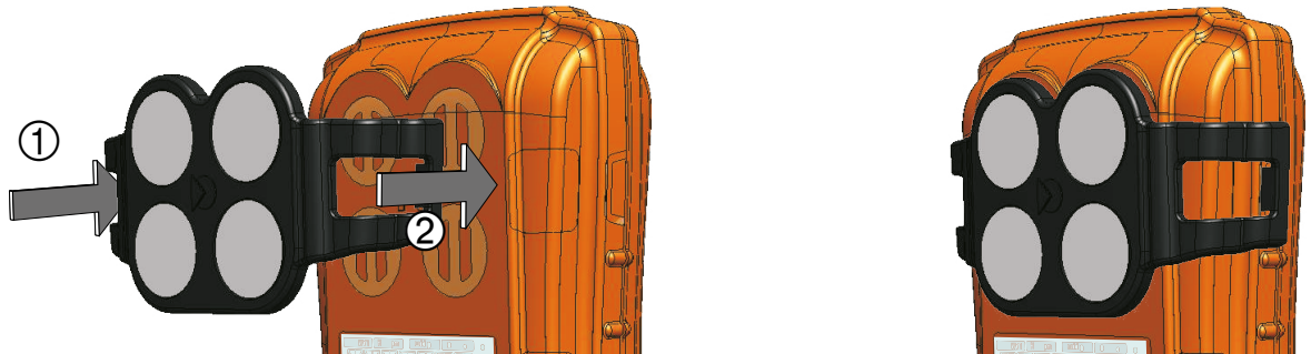
Figure 6: Fitting the external filter plate
