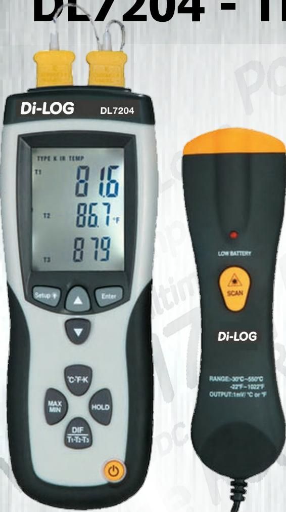
The DL7204 is a hand held Digital Thermometer supplied with an attachable Non Contact Infra Red probe. With dual K-Type input and data logging, the DL7204 is the ultimate temperature meter for advanced applications
