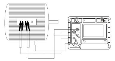
(9) Disconnect the test leads from the motor, start the motor.
