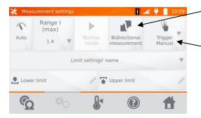
Switching Unidirectional/Bidirectional measurement.
