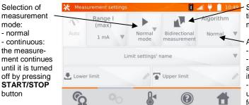
Switching Unidirectional/Bidirectional measurement.
