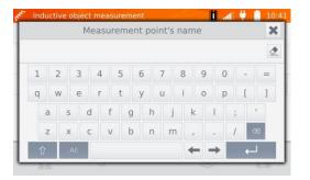
When necessary, name the measuring point.
