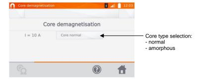
Connect the meter to the transformer windings. Press START/STOP. Wait for the following screen.
