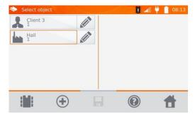
After adding and saving the object (also subobjects if necessary), click button to add the measurement point.
