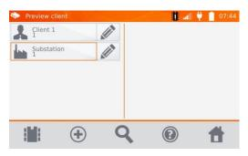
Click of the client, and then for press button at the level of the object (subobject).
