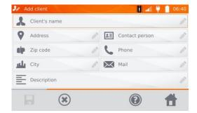
By clicking the individual fields, enter customer data using the keyboard. Client's name (box marked in orange) is mandatory.
