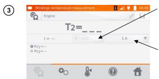
The method of supplying the measuring current is non-adjustable and set on Auto mode - the measuring current is limited to a value not exceeding the set value.
