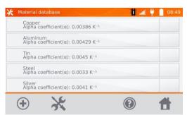
The meter has 5 defaults materials saved in the memory, together with the thermal resistance coefficients of: copper, aluminium, tin, steel and silver. Use button to add a new material.
