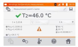
$R_{\text{T1}}$  – resistance of the cold winding
