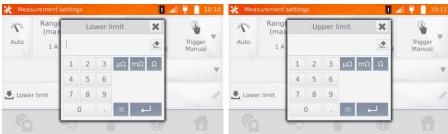
6 Click button to enter the temperature settings. After checking "Temperature compensation" box, the meter uses the specified temperatures and temperature coefficient of resistance to calculate the resistance at the reference temperature.
