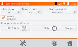
Uncheck **Screen keyboard** box to inactivate the screen keyboard.
