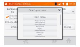
Click the selected startup screen (the screen will be automatically shown after turning on the meter). This feature is useful for making measurements of a given type for a longer period.
