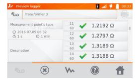
When using the logger, clicking the field with results will cause the meter to display the individual samples. You may scroll them using , buttons. Use button to display the graph.
