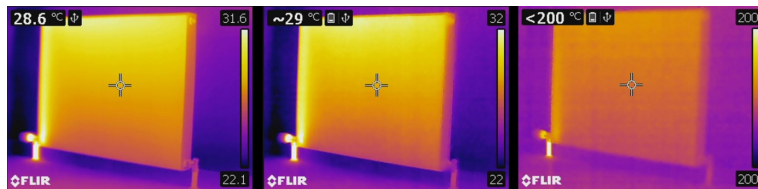
Figure 16.4 Images from a FLIR T440 with temperature ranges of -20 to +120^{\circ}\text{C} , (left, -4 to +248^{\circ}\text{F} ) and +250 to +1200^{\circ}\text{C} (right, +482 to +2192^{\circ}\text{F} ). All other settings are unchanged.
