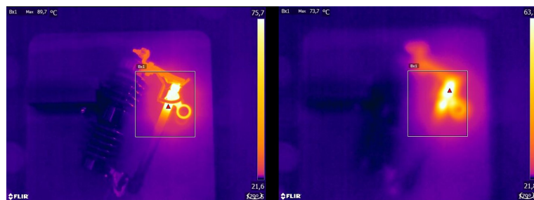
Figure 16.2 Focused thermal image (left) with a maximum temperature of T_{max} = 89.7^{\circ}\text{C} ( 193.5^{\circ}\text{F} ) and an unfocused thermal image (right) with a maximum temperature of T_{max} = 73.7^{\circ}\text{C} ( 164.7^{\circ}\text{F} ).
