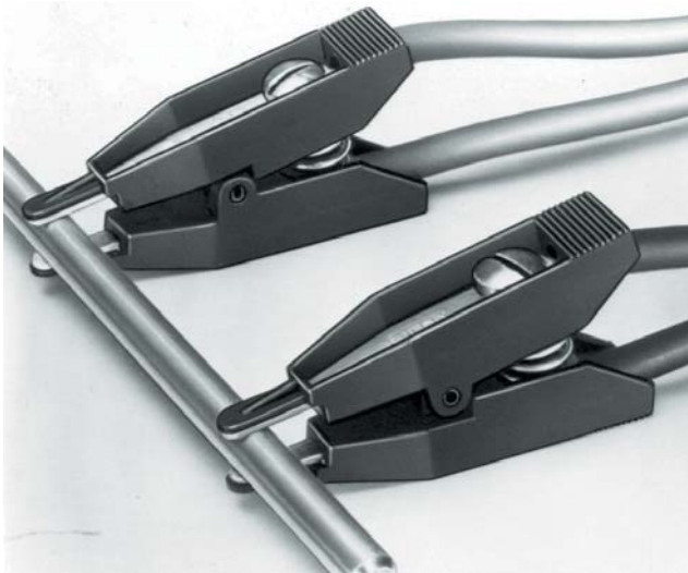
Fig. 8.2 Combined current and potential probes
