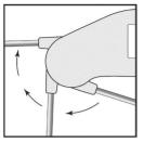
damage will occur. It is recommended to store the probe, in the closed position, when not in use.
