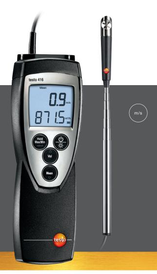
The testo 416 is a compact anemometer with a fixed vane probe. The measuring instrument is particularly suitable for flow velocity measurements in ducts thanks to the extendable telescope (max. length 890 mm, diameter 16 mm). The volume flow is directly shown in the display. For volume flow calculation purposes, the duct cross-section area can be conveniently entered into the testo 416. The timed and point mean value calculations provide information on the average volume flow.
