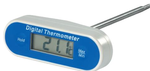
**INSTRUMENT OPERATION** - The instrument is switched on by pressing any function button located on the front of the thermometer. Apply the tip of the probe to the substance or medium to be measured. The instrument reading may take a few seconds to stabilise, depending on the nature of the measurement. The instrument will automatically turn off after 10 minutes.
