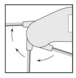
Apply the tip of the probe to the substance, surface or area to be measured. The probe should be allowed adequate time to stabilise to the temperature of the item to be measured.
