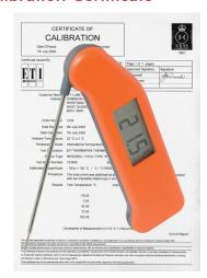
Should you require full UKAS Calibration Certification for your Thermapen, this can be supplied. Each UKAS Certificate indicates the deviations from standards at various check points -18 °C, 0 °C, 40 °C, 70 °C and 100 °C with a guaranteed uncertainty of 0.15 °C.
