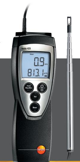
testo 425 is a compact anamometer with a fixed thermal flow velocity probe. The probe head has a diameter of 7.5 mm. With the extendable telescope (length max. 820 mm), the measuring instrument is suitable for flow velocity measurement in ducts. The testo 425 also measures extremely accurately in the low flow velocity range. The volume flow is directly shown in the display. For the purposes of volume flow calculation, the duct area can be
