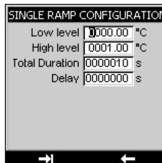
Use the **F2** key to access the **CONFIGURATION/RAMP** menu. Attention: the appropriate function mode must be programmed (**INCREASES** mode) to access the **CONFIGURATION/RAMP/SINGLE** menu.
