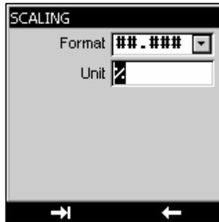
Once the parameters have been set, the scaling is automatically enabled. To disable it, enter the **Configuration/Scaling** menu, select **OFF** and confirm by pressing the **VAL** key.
