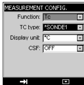
Note: the Calibrated sensors are at the top of the list and their name is preceded by a \*.
