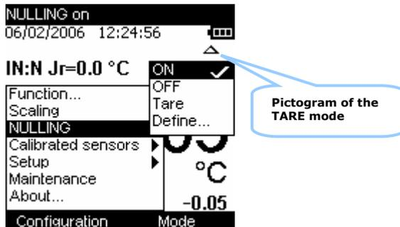
The **NULL/define** menu makes it possible to program the value of the Tare (positive or negative). This value is obtained from the measurements:
