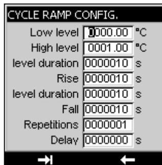
Use the **F2** key to access the **CONFIGURATION/RAMP** menu. Attention: the appropriate function mode must be programmed (**Single Ramp** mode) to access the **CONFIGURATION/RAMP/CYCLIC RAMP** menu.
