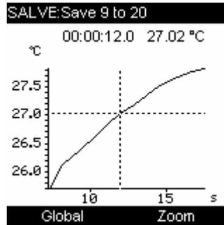
At this level, you can display the whole curve or a zoom around the cursor. The cursor is moved using the navigation keys(← and →)
