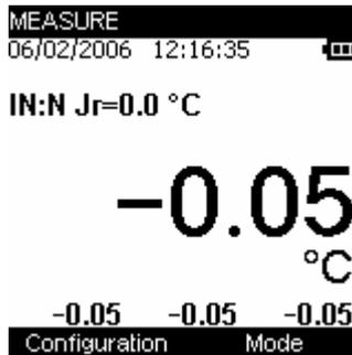
The **Measurement** mode makes it possible to display the Min (bottom left), Average (bottom centre) and Max values (bottom right) from the last **RAZ Min/Max** command.
