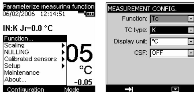
In the **CONFIGURATION MEASURE (MEASUREMENT CONFIGURATION)** menu, position the cursor in the **thermo couple** field using the **F1** key.
