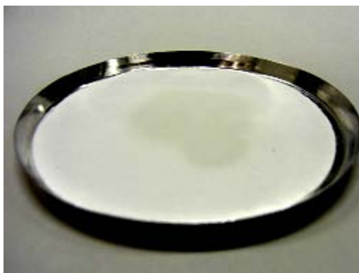
1 g milk distributed evenly via a fiber glass filter
