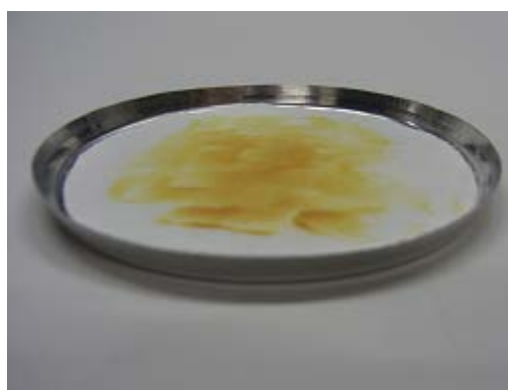
Water and oils evaporate, minor discoloration
