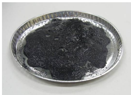
Melted with encrusted surface
