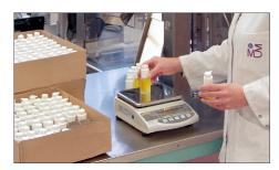
Weighing with tolerance range (check-weighing): a visual signal helps with portion division, dispensing or grading
