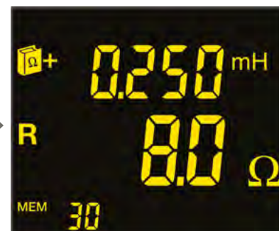
Screen 3: value of the the resistive and inductive part of the impedance measured
