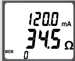
Screen 1: Impedance and leakage current
