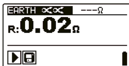
Figure 5.8: Example of contactless earthing resistance measurement result
