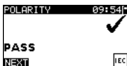
Figure 1.61: Polarity test result screen
