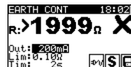
Figure 1.27: Examples of Earth continuity resistance measurement results
