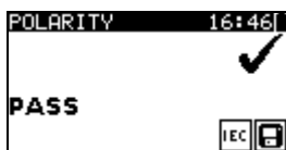
Figure 1.42: Examples of polarity test result
