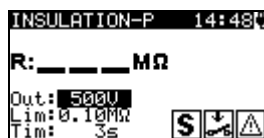
Figure 1.31: Insulation resistance - P menu
