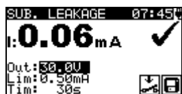
Figure 1.36: Example of substitute leakage current measurement results
