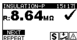
Figure 1.57: Insulation resistance - P result screen
