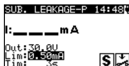
Figure 1.58: Substitute leakage - P starting screen
