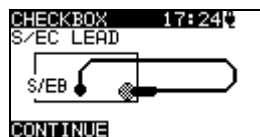
Figure 1.16: S/EB test lead check starting screen
