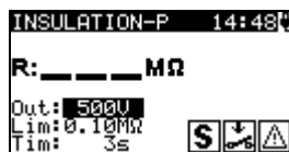
Figure 1.56: Insulation resistance - P starting screen
