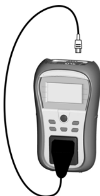
Figure 1.41: Polarity test of IEC cord
