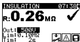
Figure 1.30: Examples of Insulation resistance measurement results
