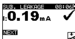
Figure 1.55: Substitute leakage result screen
