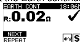
Figure 1.51: Earth continuity result screen
