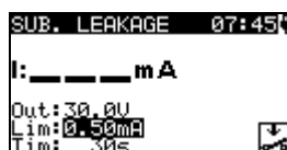
Figure 1.54: Substitute leakage starting screen
