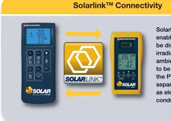
Solarlink<sup>™</sup> connectivity enables irradiance to be displayed and for irradiance, module and ambient temperature to be recorded with the PV150 (available separately) in real time as electrical tests are conducted.
