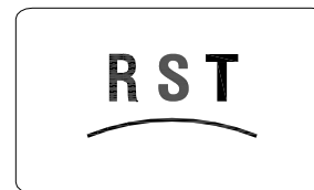
Figure 15 Any phase of voltage is less than 30V.
