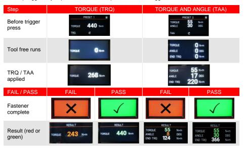
If fastener was releasing final torque will be zero.
