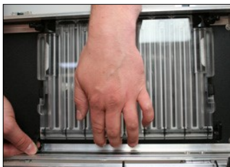
Fig. 65: Refitting the condenser
