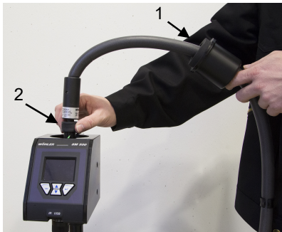
Fig. 84: Disconnecting the heated sample intake hose
