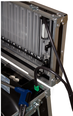
Fig. 56: Probe and cable-hose assembly connection for flue gas analysis
