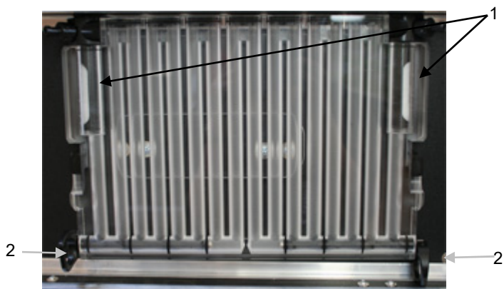
Fig. 62: Close-up view of the flue gas condenser
