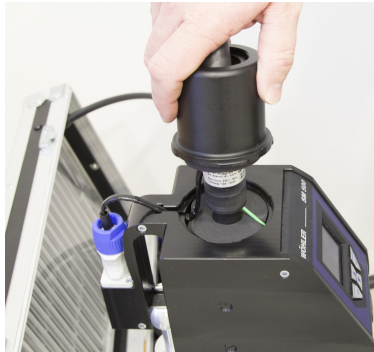
Fig. 90: Connection cable of the heated sample intake hose routed according to best practice
