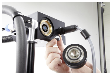
Fig. 9: Changing the filter
