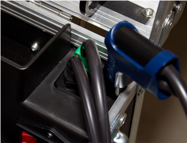
Fig. 60: Probe and cable-hose assembly connections for draft measurements
