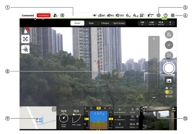
Fig 3-24 Interface layout (camera interface)
