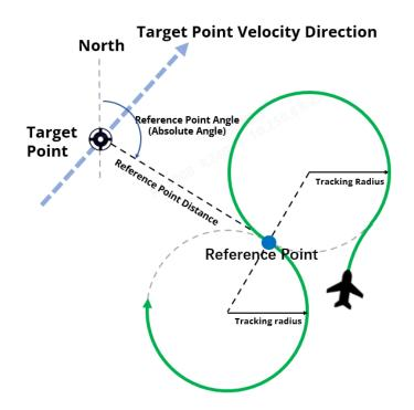
Fig 4-38 Figure-8 circling tracking
