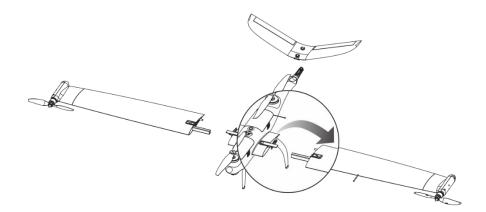
Fig 4-1 Install the wings
