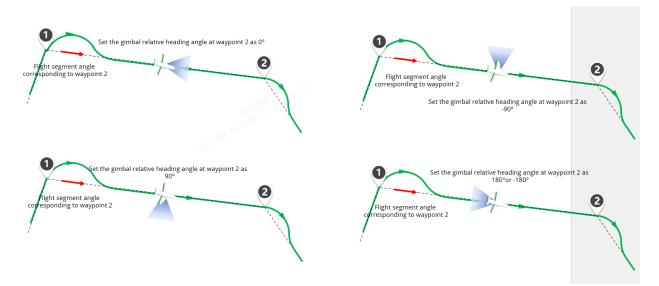
Fig 4-23 Description of gimbal relative heading angle
