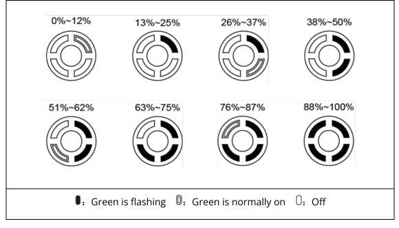
Fig 3-5 Battery level indicator status (non-charging status)
