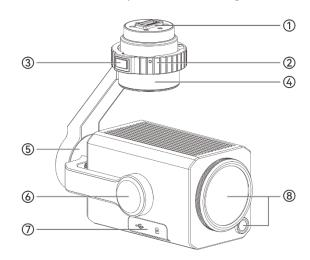
Fig 3-8 Gimbal structure (DG-Z2 as an example)
