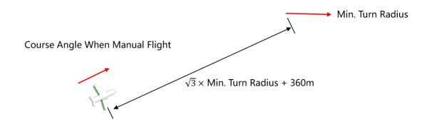
Fig 4-53 Position of arrival hovering point in return in manual flight
