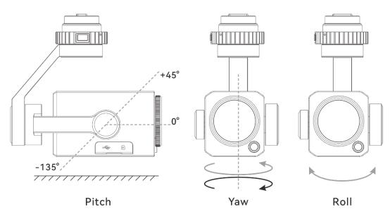
Fig 3-10 Description of the mechanical rotation range of the gimbal (the picture above shows the DG-Z2)
