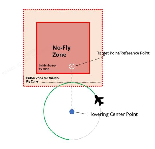
Fig 4-16 When the target point is inside the No-fly zone
