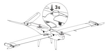
Fig 4-4 Aircraft powering on
