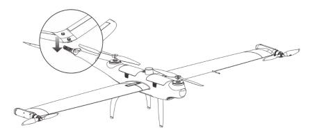
Fig 4-2 Install the rear wing
