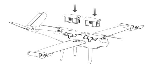
Fig 4-3 Install the Smart Battery
