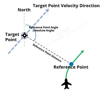
Fig 4-39 Synchronous tracking
