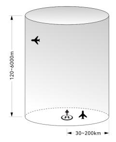
Fig 2-7 Diagram of altitude and distance limits
