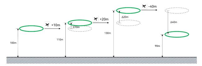
Fig 4-47 Change altitude logic multiple times with one click
