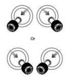
Fig 4-29 Start The Aircraft Motor
