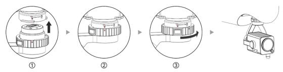
Fig 3-11 Install a gimbal camera on the aircraft
