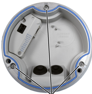
Twist-lock screws in back box
