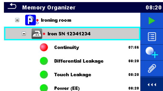
Figure 5.6: Status - Measurements completed with fail result(s)
