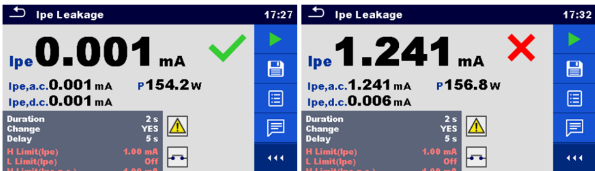
Figure 6.50: Examples of Ipe Leakage measurement results
