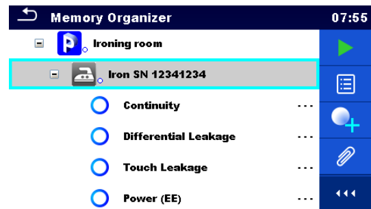
Figure 5.4: Example of status - No measurement result(s)
