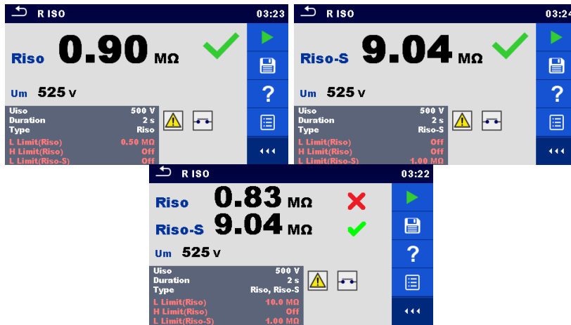
Figure 6.39: Examples of Insulation resistance measurement results
