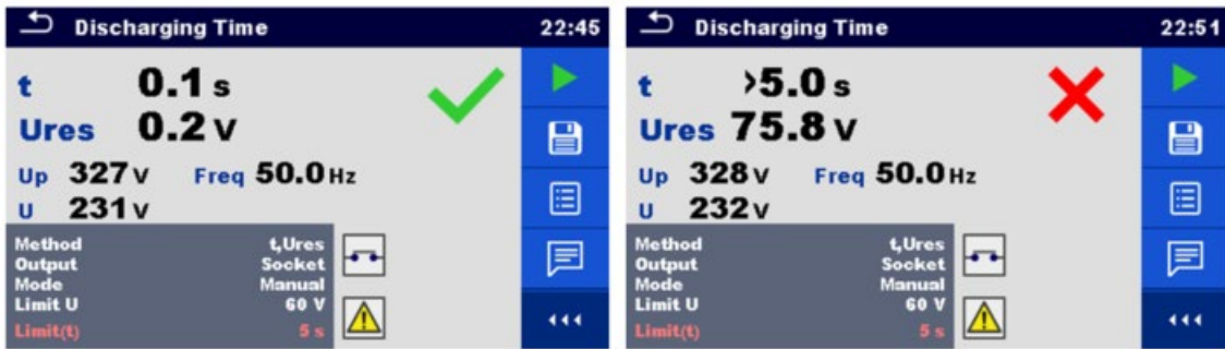
Figure 5.53: Examples of Discharging Time measurement results (Output = Socket)
