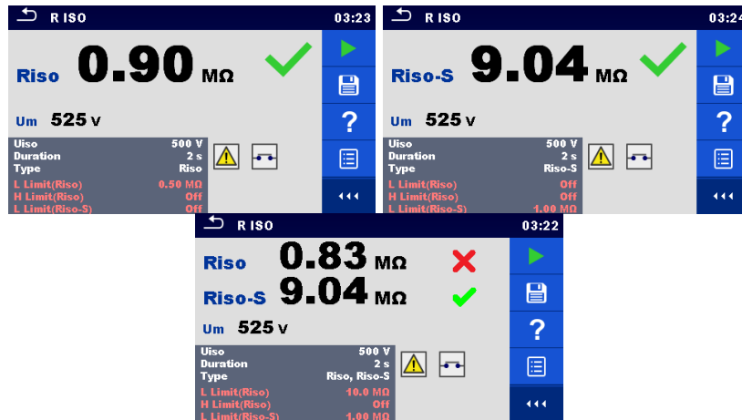
Figure 5.27: Examples of Insulation resistance measurement results
