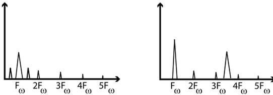
**Figure 13.2** Graph on left shows a loose equipment issue (additional frequencies near the fundamental); Graph on right shows an impulse vibration (between 3rd and 4th harmonic) . Frequency of the impulse will vary from machine to machine (speed, size, etc.).
