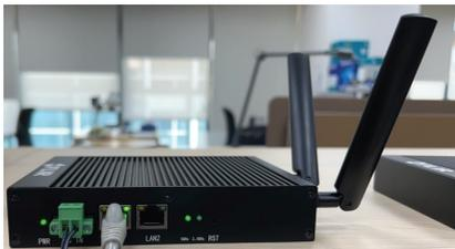
**Figure 9.2** Connecting an Ethernet cable to the GW66.
