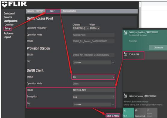
Figure 9.1 Connecting to the 5 GHz Wi-Fi Network.
