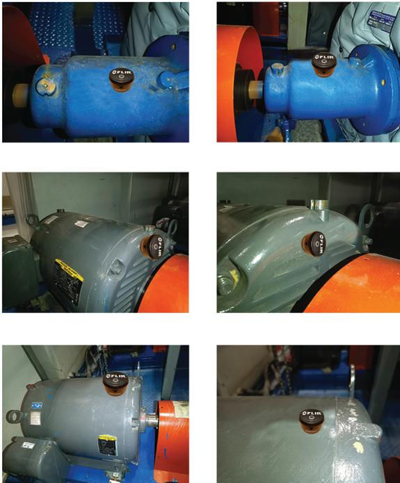
**Figure 10.2** Sensors shown mounted on machinery.
