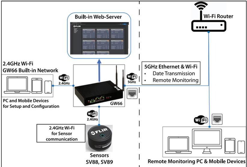
**Figure 5.1** System Architecture.
