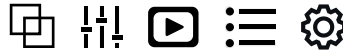
Figure 6.1 Main Menu icons (L to R: Image Mode, Thermal Settings, Gallery, Advanced Menu, Settings)
