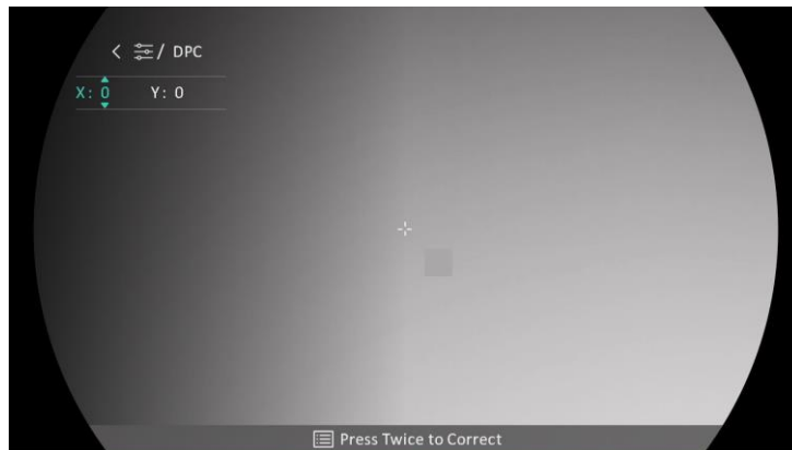
Figure 3-5 Correct Defective Pixel
