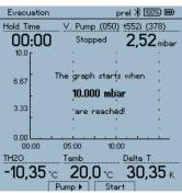
The measurement is running, the vacuum holding test has not yet started.
