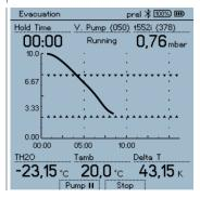
When the target values are reached, the evacuation and therefore also the pump are stopped automatically.
