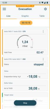
The measurement data is transferred to the testo Smart App and evaluated there.
