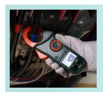
Clamp meters with built-in non-contact infrared thermometer
